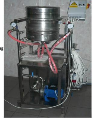
After complete sterilization, the keg is CO<sub>2</sub> purged and pressurized, and is ready for filling.
